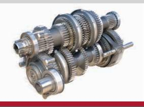
The right speed for each job is conveniently selected using gear levers that are within easy reach, yet positioned neatly to the driver's hand, ensuring an unimpeded passage when mounting/dismounting. A single-plate, wet clutch is easy to operate and simple to service. Super Creeper option is also available when the lowest speeds, down to .08 MPH\*, are required for the job at hand.
