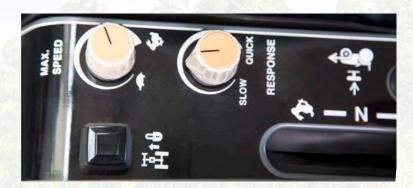
**CRUISE CONTROL FEATURE IS STANDARD** — With the hydrostatic transmission and lets you set a precise working speed — just engage and go. Pressing the brake pedal or the forward pedal disengages the system.
