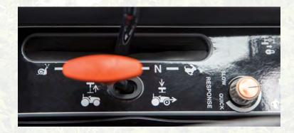
**GET EXTRA TRACTION FOR TOUGH JOBS** — And difficult conditions with on-demand four-wheel drive. Just push the lever downward to engage, pull it up to disengage.
