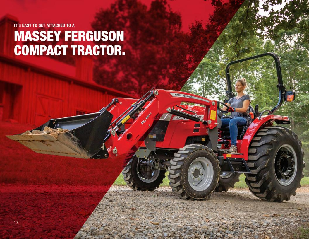
START WITH THE FL SERIES LOADER — It's available with a 66- or 72-inch width bucket. The standard skid-steer coupler makes it easy to remove or hook up the bucket. Add a third diverter — and get the versatility of other popular skid-steer attachments — such as a grapple or 4-in-1 bucket.
