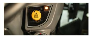
A STANDARD 540 RPM REAR PTO AND OPTIONAL 2000 RPM MID-MOUNT PTO ARE ELECTROHYDRAULICALLY CONTROLLED
