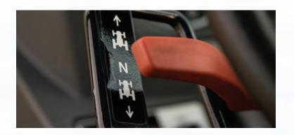
A HANDY SHUTTLE-SHIFT LEVER — Lets you change direction fast and easy — ideal for loader work, and located on the steering column.
