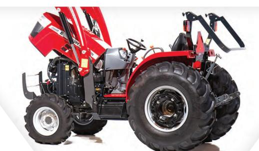
**THE STANDARD FOLDING ROPS** allow an MF E Series to fit beneath a standard 7-foot garage door.
